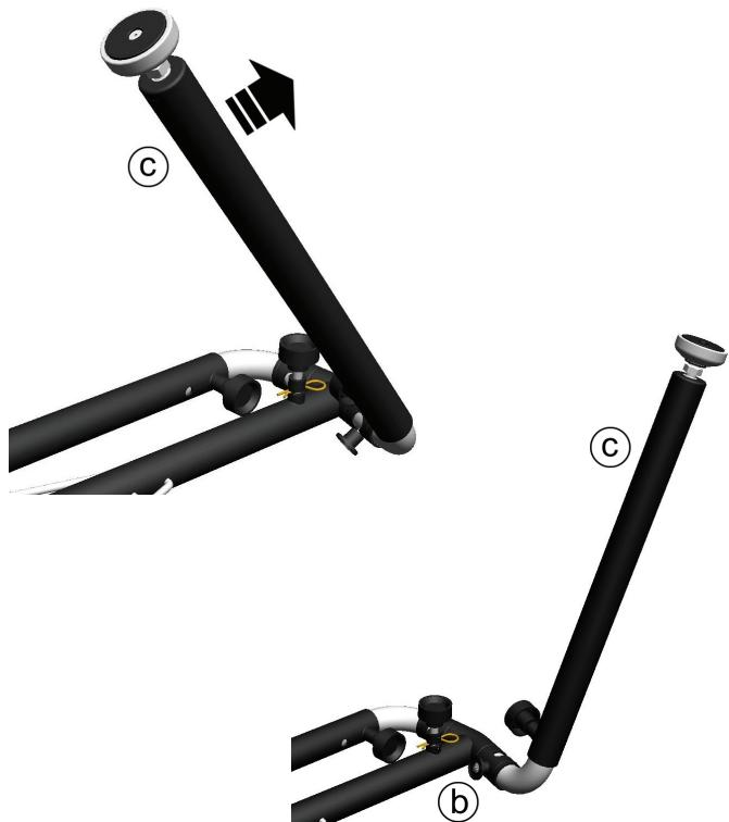
5. Untighten the screw (d), and slide out the movable part of the leg (c').
