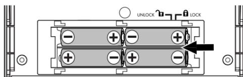
1. Slide the cover of the battery case in the direction of the arrow, and open the cover.
