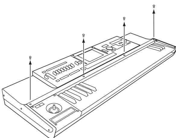
4. Raise the module slightly, and then use both hands to lift it up, removing the module and retaining bar "A" from the keyboard assembly.
