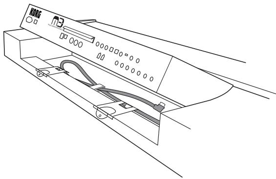
3. Using your Philips (+) screwdriver, remove the four screws from retaining bar "A" that holds the module to the keyboard assembly.
