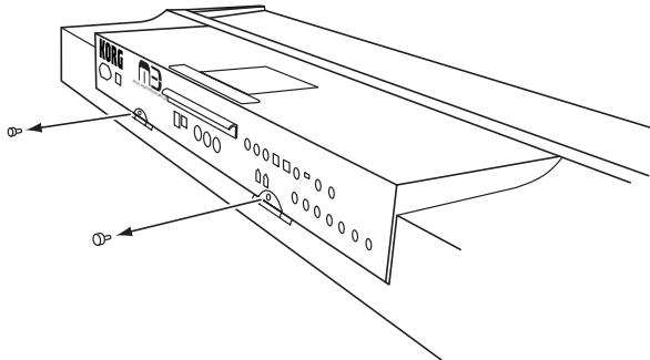
2. Grasp the handle affixed to the module's rear panel, and gently tilt the module up.
