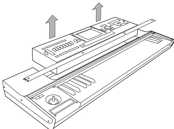
5. Re-attach the retaining bar "A" using the screws you removed in step 3. This will keep the screws and retaining bar "A" safe for future use.
