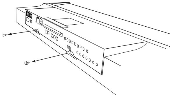
2. While using one hand to raise the module, unplug the cable (the "L" shaped plug) that's connected to the TO KYBD connector on the bottom of the module, and gently lower the module.
